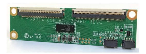
YW52H4564P5656 Controller Board was developed based on WDT8752A. WDT8752A is Touch Controller with an enhanced analog front end (AFE) and digital front end (DFE) circuit including an HV charge driver on multi-touch capacitive panels.
